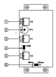
(1) AC/DC POWER SUPPLY Power supply terminal block connector.
